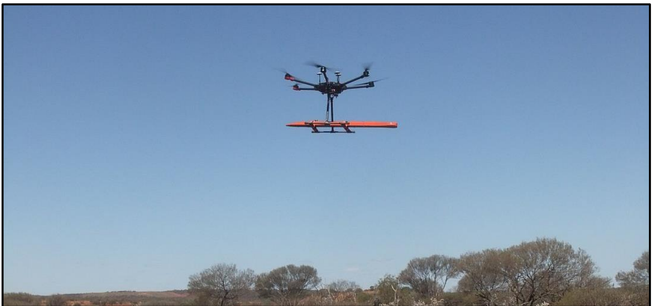
Figure 6. UAV (unmanned aerial vehicle) conducting magnetic geophysical surveys.
